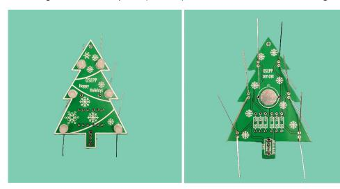
STEP 2: Place and solder the resistors into place.
